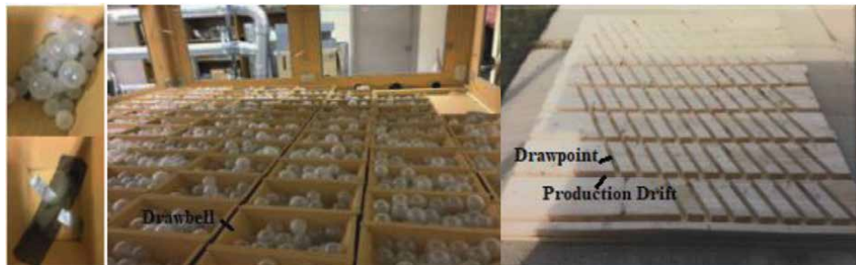
Figure 29. Arrangement of drawbells and drawpoints with an El Teniente layout.
