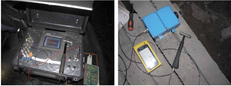
Figure 8. The portable measurement system for quality control of installed rock bolts, working prototype (left) and final version fulfilling ATEX requirements (right).
