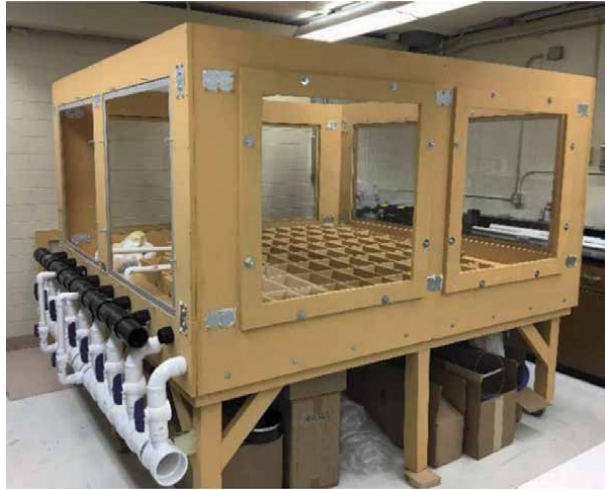
Figure 28. Experimental model showing production drift inlets.
