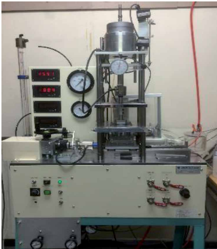
Figure 2. Direct simple shear test apparatus.
