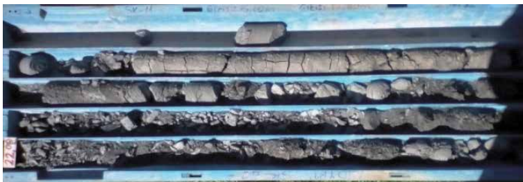
Figure 5. Shale and alluvium logs of south steep slope faces of Avgamasya No 1 pit survey area.
