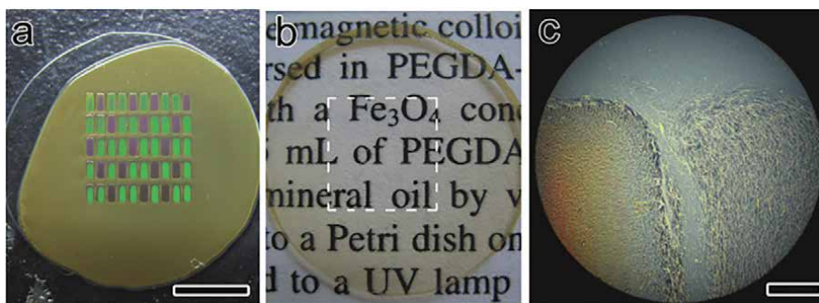
Figure 26. (a) Colorimetric binary codes array and (b) an invisible replica printed with an orientational printing process. (c) Optical microscope image of two neighboring code chips in part b. scale bars: (a, b) 5 mm and (c) 200 \mu\text{m} .
