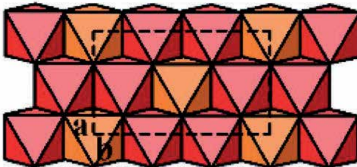
Figure 3. Arrangement of octahedral unit to form the octahedral sheet.
