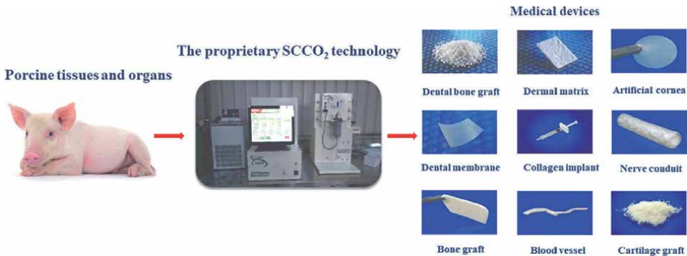
Figure 3. Production of collagen scaffolds by SCCO 2 technology.
