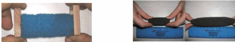
Figure 2. Usually used test-demonstration of auxeticity.
