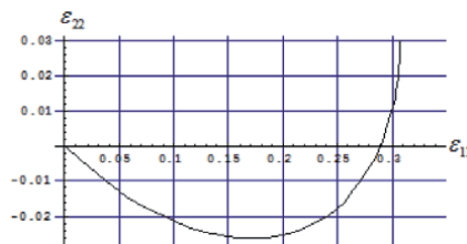
Figure 20. Dependence of longitudinal and transverse strains (polystyrene).
