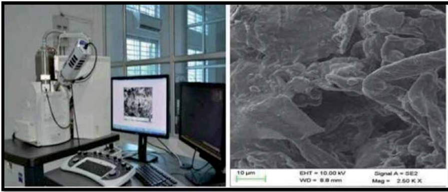
Figure 15. FESEM image for pulp ratio and epoxy resin for composite sheet.
