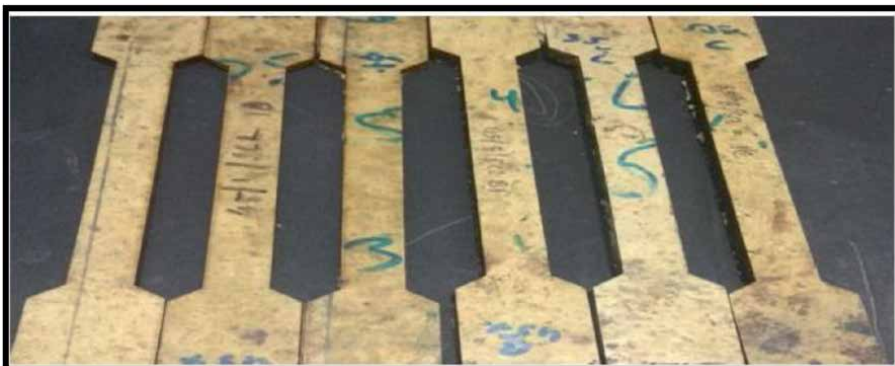
Figure 10. Specimen size for composite sheet material.
