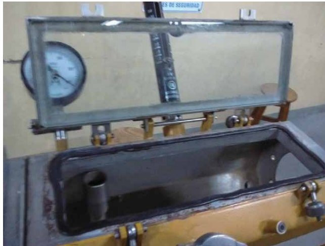
Figure 19. Cooling and vacuum calibration pan.
