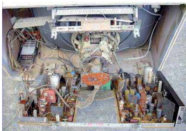
Figure 3. Digital TV receiver contains Mn-ferrites deflection yokes [15].
