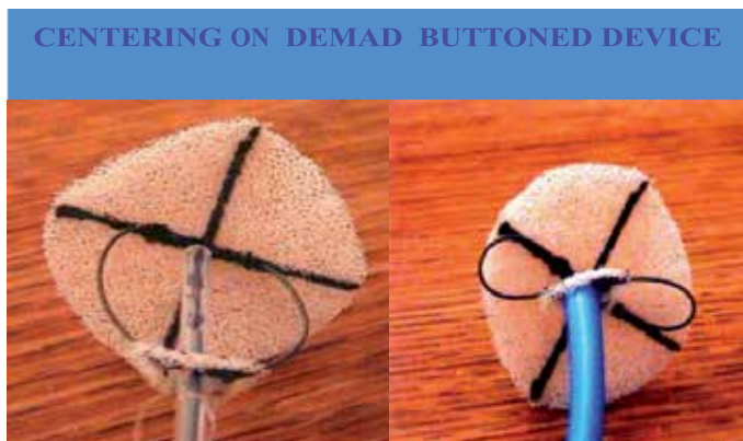
Fig. 9. Photographs of centering on demand buttoned device with the centering mechanism open (left panel) and closed (right panel).
