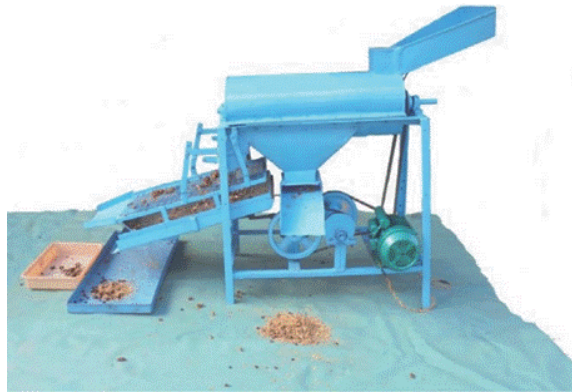
Figure 7. Tamarind dehuller developed at Tamil Nadu Agricultural University, Coimbatore.
