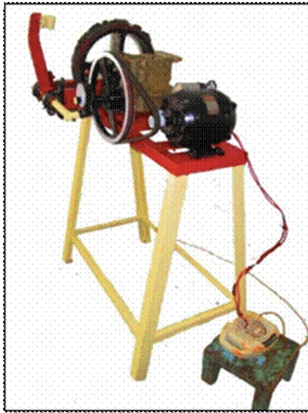
Figure 10. A hammer-type tamarind deseeder is available at Tamil Nadu Agricultural University.
