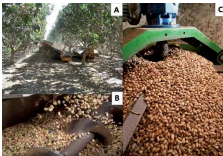
Figure 4. Harvesting and post-harvest processing of pistachios in California: (A) off-ground harvesting [43]; (B) mechanical dehulling; (C) cylindrical hot air drying.
