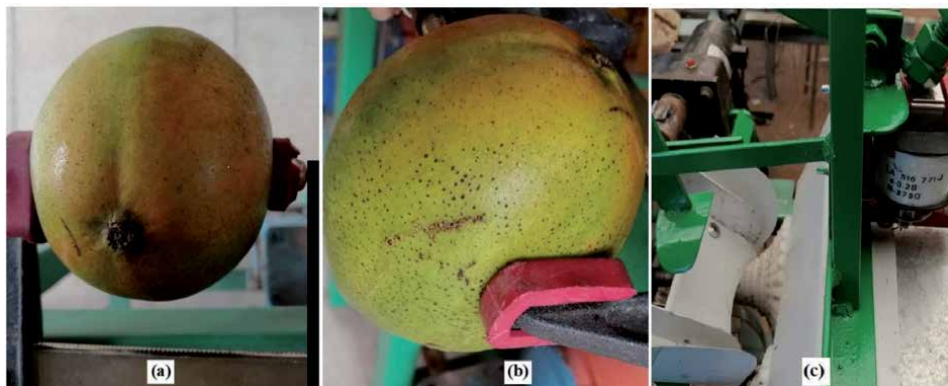
Figure 2. Robotic gripper (a) with mango pedicel, (b) without mango pedicel and having wounds, (c) cauterizer knife machine.
