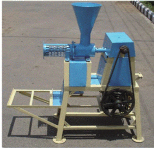
Figure 9. Tamarind deseeder developed at Tamil Nadu Agricultural University, Coimbatore.
