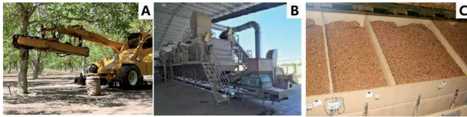
Figure 3. Typical harvesting and postharvest processing of walnuts: (A) walnut shaking; (B) hulling and washing section; (C) hot air drying bins.
