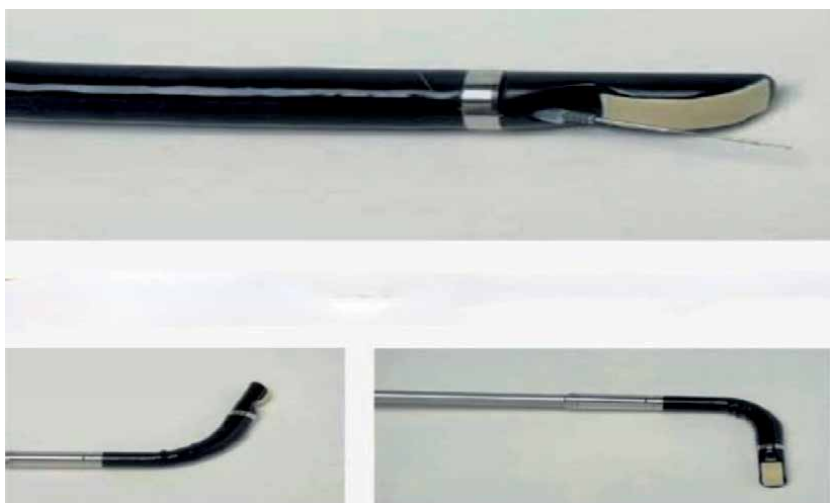
Figure 2. (a-c) A laparoscopic probe has a needle biopsy enhancement (a, above) and two lower images (b, c) showing the flexibility of the tip of the probe.
