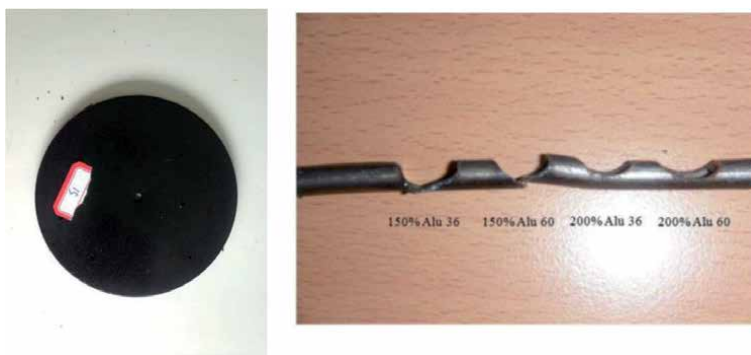
Figure 13. Left: example of angle grinder disc formed by a tannin-furfuryl rigid plastic matrix and aluminium oxide abrasive. Right, example of a steel tube cut with the same type of disc but with different abrasive grits [72].
