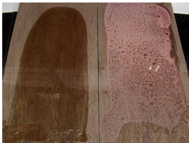
Figure 6. Appearance of cured films of DA-1 (left) and moisture cured PUR control (right).
