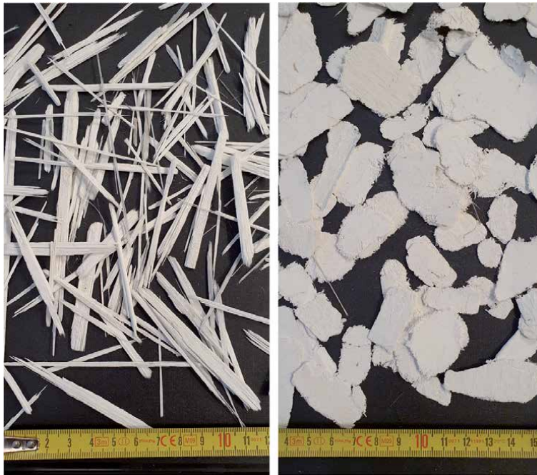
Figure 5. Shreds from rotor blades (left) and from boat hulls (right).
