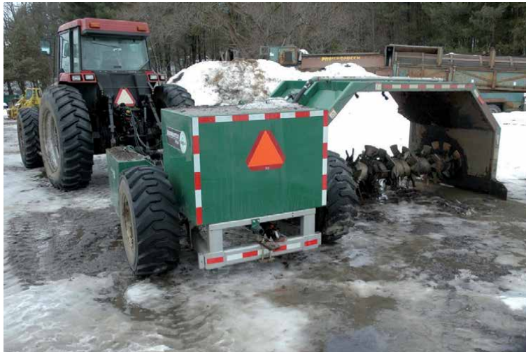
Figure 8. This mechanized device is pulled by a tractor and is used to shape, turn, or churn the compost in the windrows.
