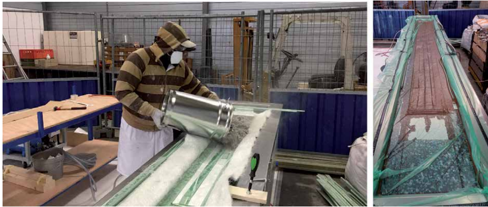
Figure 10. Production of profiles using EoL composite by vacuum infusion under foil [3].
