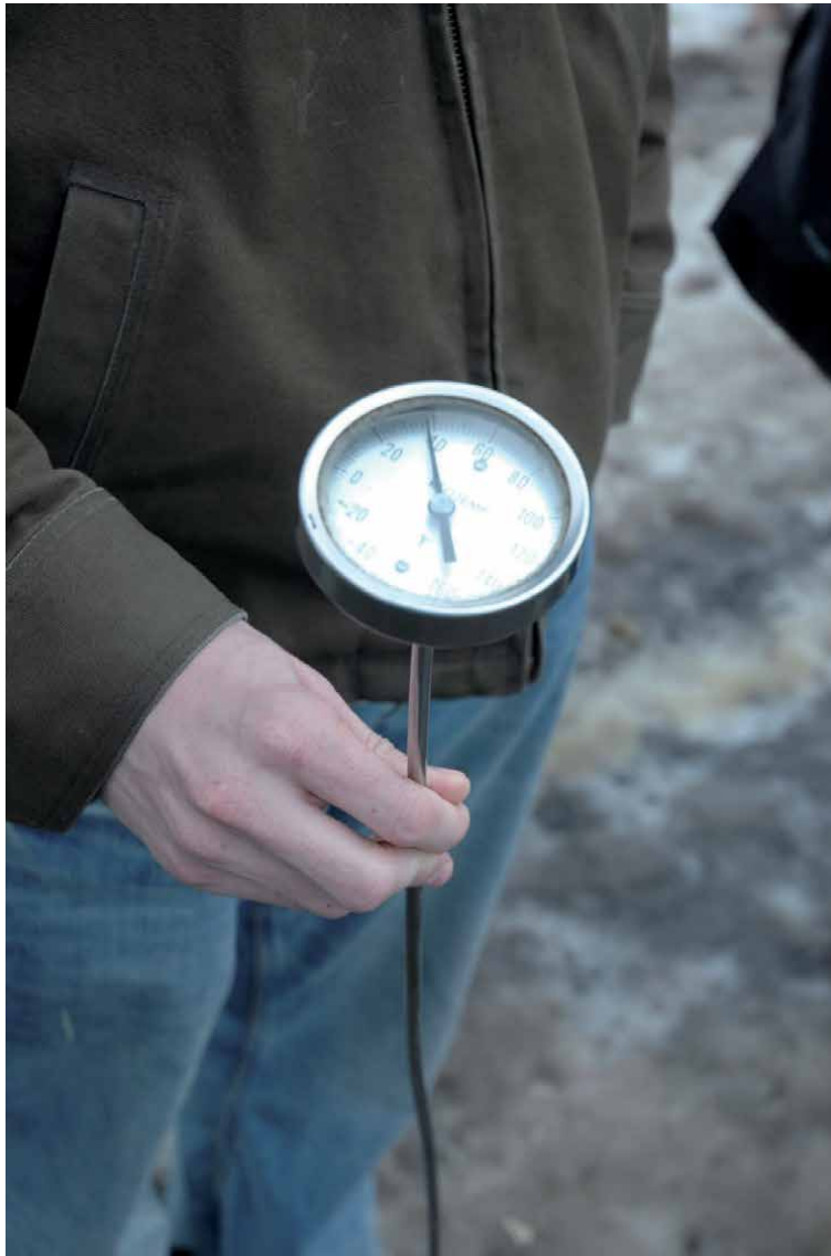
Figure 12. Decomposition temperature is monitored regularly using this thermometer with a 1 meter long probe.
