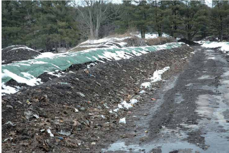
Figure 7. This is an example of a municipal compost facility using wind-rows for large-scale production.
