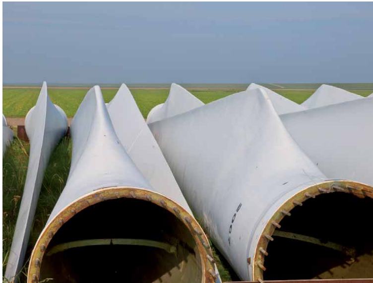
Figure 1. Obsolete windmill rotor blades [3].
