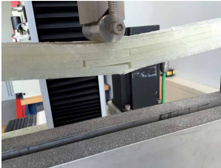
Figure 7. Bending test of a specimen made with 80 mm strips [4].
