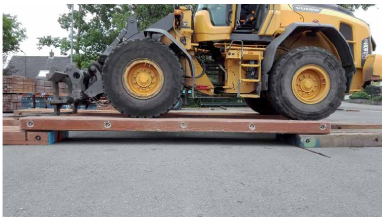
Figure 14. Crane mat made of EoL composite tested in practice [3].
