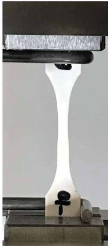
Figure 1. (a) Schematic of an ASTM tensile bar (type V) 6 and (b) experimental set-up.
