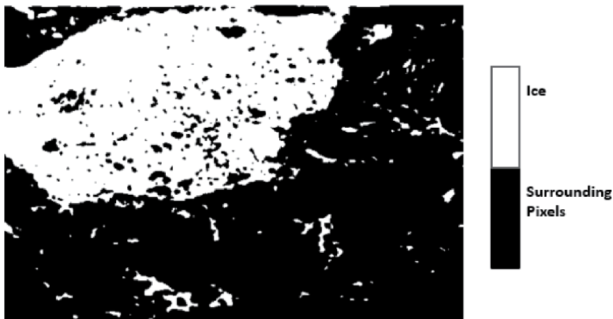
Figure 5. Automatic detection of ice covers in SAR data using MBGA.
