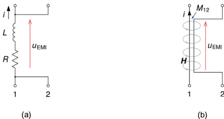
Figure 5. Equivalent circuit: Galvanic coupling (a) and inductive coupling (b); R – Resistance, L – Self-inductance, M_{12} – Mutual inductance between wires, i – Disturbing current, u_{EMI} – Disturbing voltage, H – Magnetic field strength.
