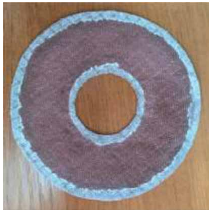
Figure 4. Same woven fabric with plasma copper coating.
