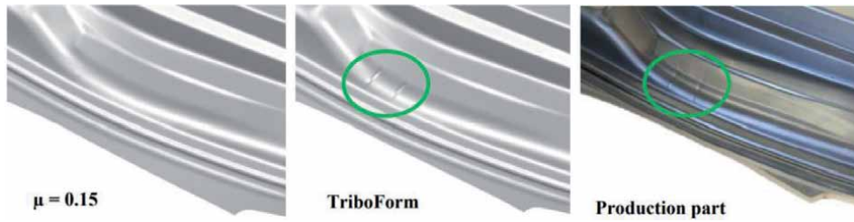
Figure 22. Simulation with constant friction and variable friction compared to a real piece. Source: Sigvant et al. [25].
