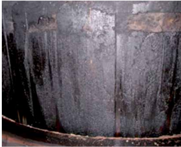
Figure 25. CaCO 3 deposits on the piston top.
