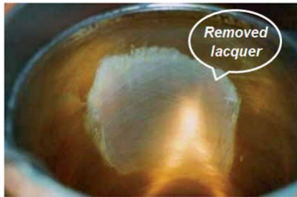
Figure 18. Liner lacquer after partial cleaning with acetic acid [17].
