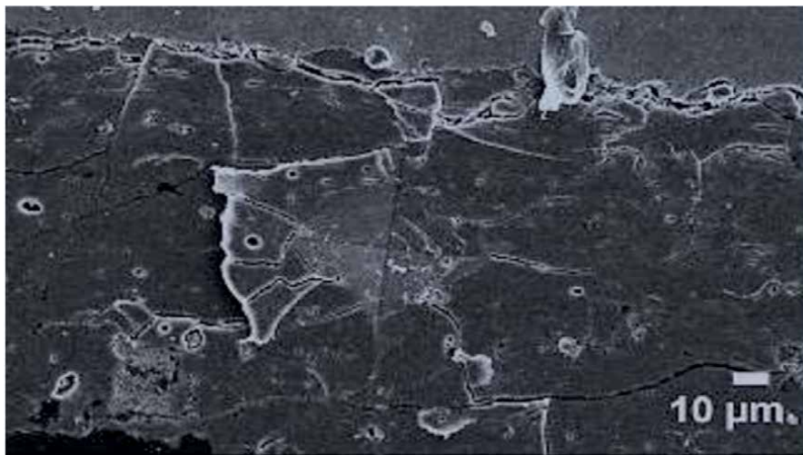
Figure 7. Radial cracks on HA-CNT coating caused by microindentation.
