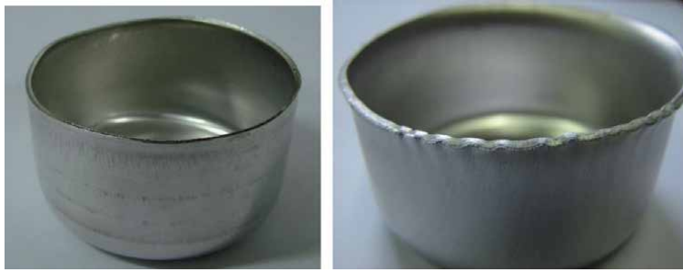
Figure 13. Pieces stamped with different lubricants under the same conditions. Left figure: Liquid lubricant. Right figure: Teflon sheet. Source: Folle and Schaeffer [6].
