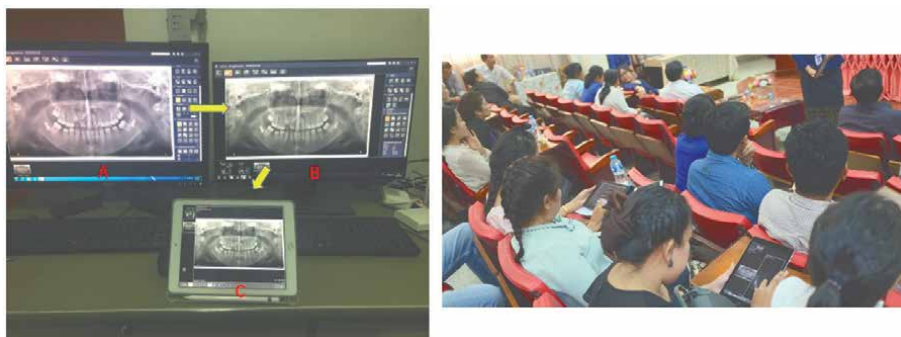
Figure 7. Medical ICT system using the tablet terminal. Left: Digital image data (A) are transferred through PC server (B) to the tablet terminal (C). Right: Workshop for dentists (teachers).
