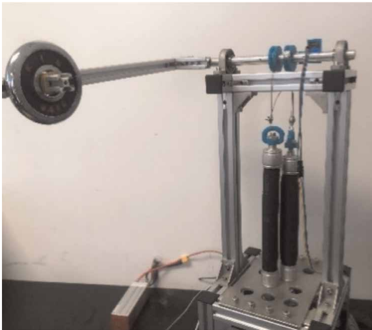
Figure 9. The experimental platform of the bionic robotic joint actuated by antagonistic PAM pair.
