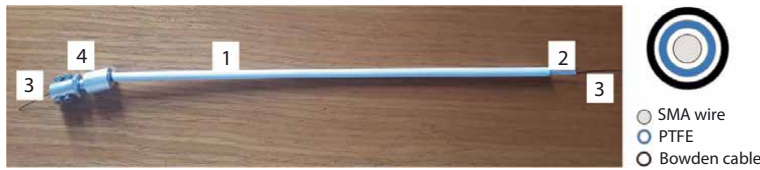
Figure 1. SMA-based actuator. Right side: 1 – Bowden cable; 2 – PTFE tube; 3 – SMA wire; 4 – Terminal unit; left side, actuator cross section.
