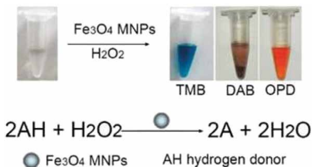
Figure 1. Iron oxide nanoparticles with peroxidase-like activity catalyze colorimetric reaction mediated by HRP [6]. Copyright 2007, Springer Nature.
