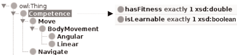
Figure 3. The competence entity with its two fundamental properties ( learnability and fitness ), modeled in the knowledge base using ontologies.
