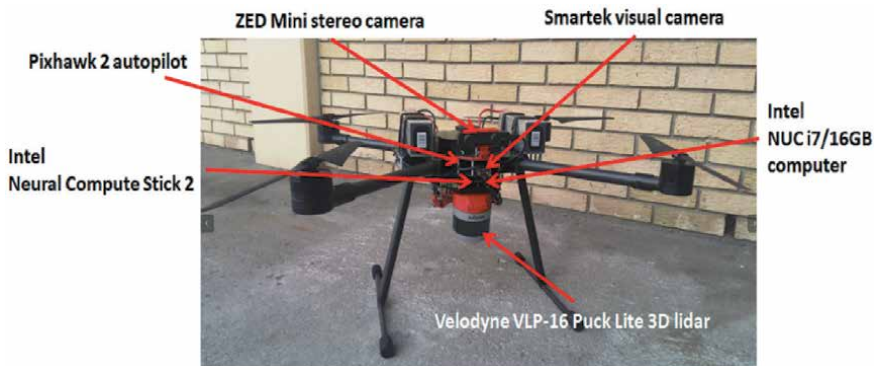
Figure 1. Front view of the aerial platform with all sensors and electronic devices on board.
