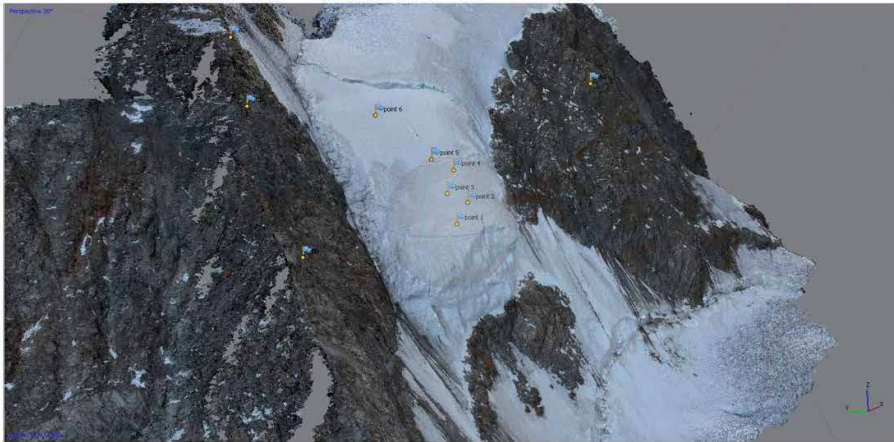
Figure 17. Point cloud rendering of the Whymper Serac obtained from a drone survey.
