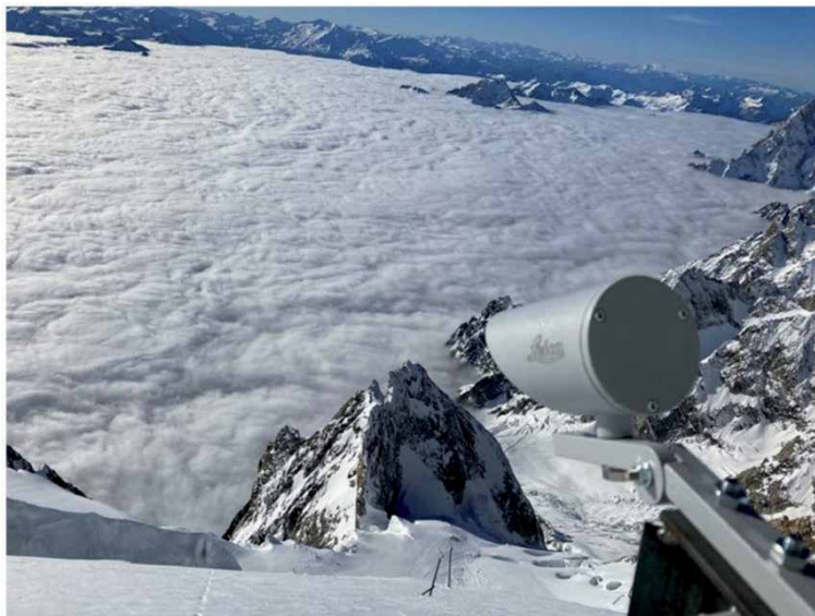
Figure 13. One of the prisms positioned on the Whymper Serac, pointing towards the robotic total station located in the hamlet of Planpincieux (photo: FMS).
