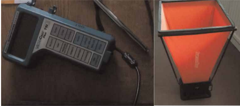
Figure 3. Ventilation measuring devices; thermo-anemometer (TSI) on the left side and airflow hood on the right side.
