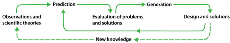
Figure 1. The iterative relationship between science and design. Observations and scientific theories are used to make predictions of the future that can be probed and tested on specific problems to generate new design solutions that either could be refined through making new predictions, or generate new knowledge that contributes to theory development. Adapted and modified from Batty [52].
