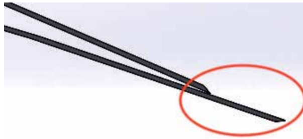
Figure 4. Trailing edge diagonal cut treatment for simplified meshing.
