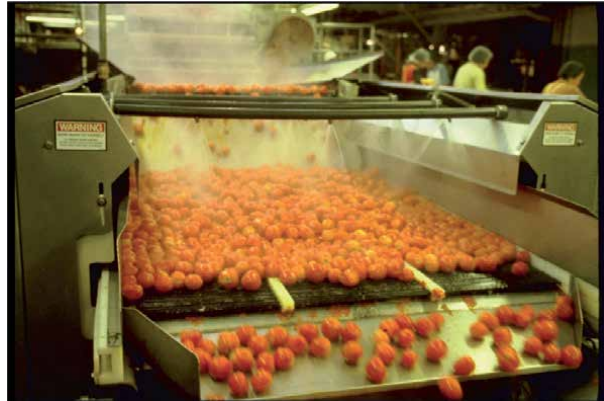
Figure 6. A disc-peeler used to separate tomato peels.
