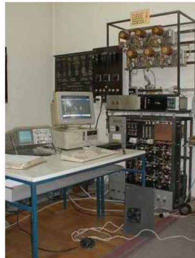
Fig. 10. CSI fed induction motor drive with improved vector control algorithm: control block diagram (left), laboratory prototype (right)
