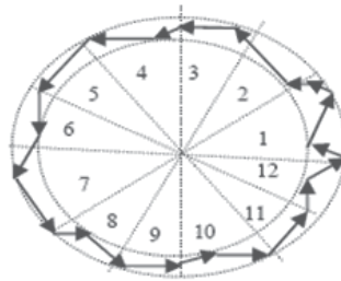
Fig. 11. Selection of vectors tensions V_s corresponding to the control of the magnitude \Phi_s for a three level inverter.
