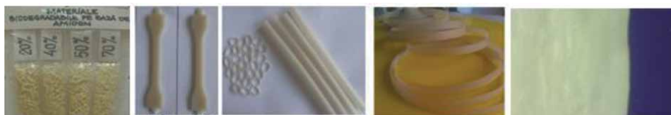
Figure 5. Granules (20–70% starch content) and items achieved from PVOH-starch compounds after elimination of defects via structuring by controlling the melt resistance to flow [17, 63].
