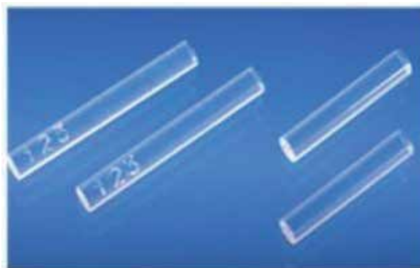
Figure 5. General type of radiophotoluminescent dosimeters (RPLDs) – glass rods.
