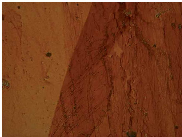
Figure 12. Optical microscopy image of graphene deposited on HgCdTe, where darker areas represent graphene on HgCdTe and lighter area portions the bare HgCdTe substrate.
