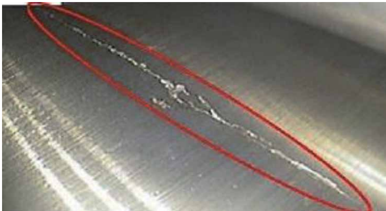
Figure 2. Inner race fault.
