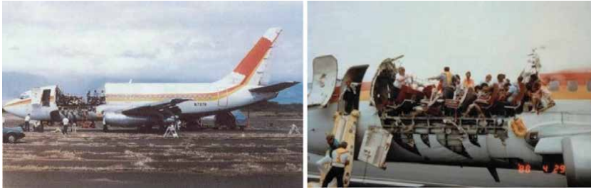
Figure 1. Boeing 737-200 fuselage fatigue failure. NTSB. Aircraft Accident Report NTSB/AAR-89/03, Aloha Airlines, Flight 243, Boeing 737-200, N73711; Near Maui, Hawaii; April 28, 1988.
