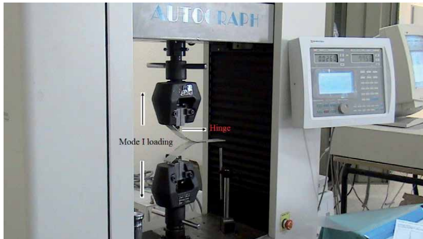
Figure 5. Experimental setup for DCB specimen and fracture in DCB test.
