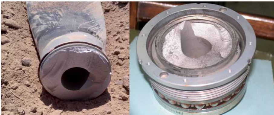
Figure 1. Fatigue failure of bonanza F33 propeller.
