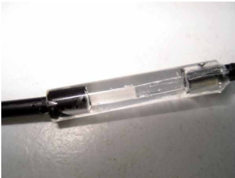
Figure 13. Optical splice with low attenuation.
