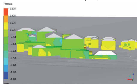
Pressure Gradient for Wind Direction: South – West (SW)
