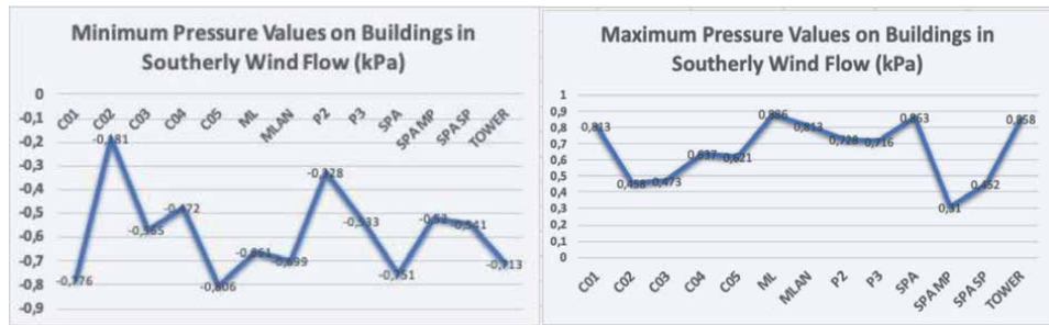
Figure 9. Maximum & minimum pressure on building facades for wind direction: South (S).
