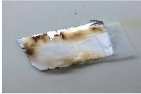
Figure 8. FOD to a chew-gum aluminium wrap which have begun a fire.
