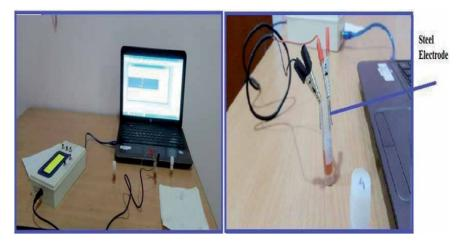
Figure 15. Measurement using steel electrode.
