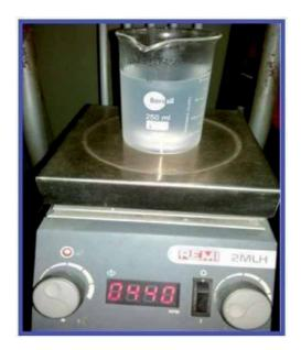
Figure 2. Zinc chloride solution is heated on a magnetic stirrer at speed 450 rpm upto 70°C.
