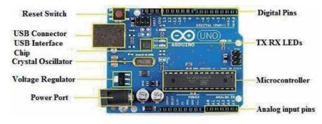
Figure 17. Arduino board.
