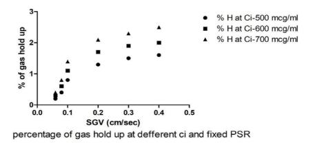
**Figure 3.** Percentage of gas hold up at defferent ci and fixed PSR.
