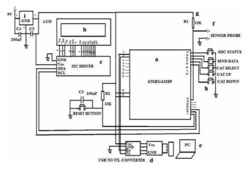
Figure 14. Circuit diagram of ZnO-NP based biosensor.
