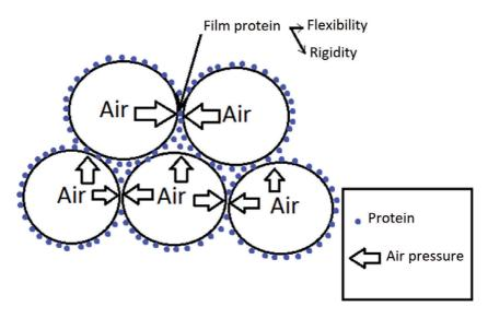
Figure 1. Schematic presentation of protein based foam.
