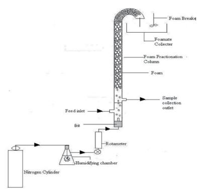
Figure 4. Schematic diagram of foam fractionation apparatus operating (batch process).
