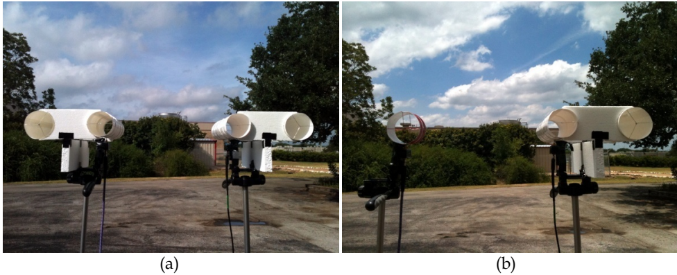
Fig. 17. Measurement setup. (a) FCH Yagi-FCH Yagi. (b) FCH Yagi-FCH dipole.
