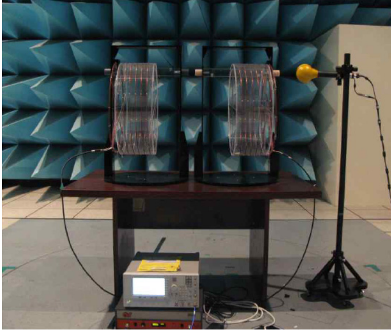
Fig. 3. WPT tested in a semi-anechoic chamber[2].
