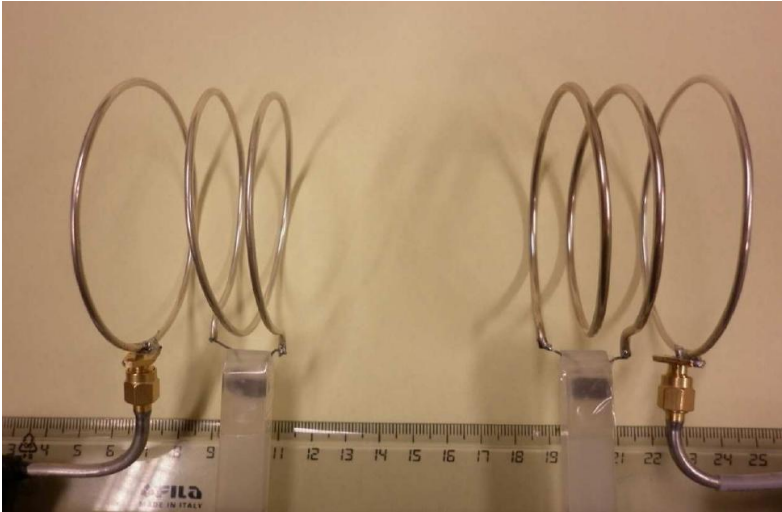
Fig. 2. A structure showing the inductive coupling between the source (first loop on the left), the transmitting resonator (second coil from the left), receiving resonator (third coil from the left) and load (last loop on the right).
