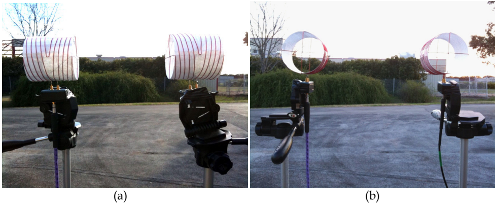
Fig. 5. Photos of the outdoor measurement setup. Each FCH is connected to a 2:1 transformer balun. (a) \theta=0 . (b) \theta=\pi/2 . ©2010 IEEE (Yoon & Ling, 2010).
