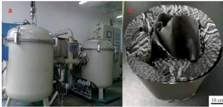
Figure 7. Optical photographs of (a) a lab-scale vacuum induction furnace and (b) roll-shaped graphite film prepared from PI film.
