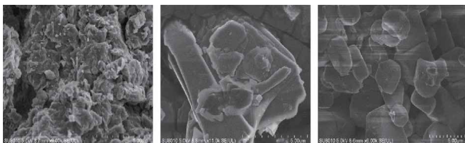
Figure 5. SEM images of the single-layered 2D mesoporous \text{TiO}_2 nanosheets [7].
