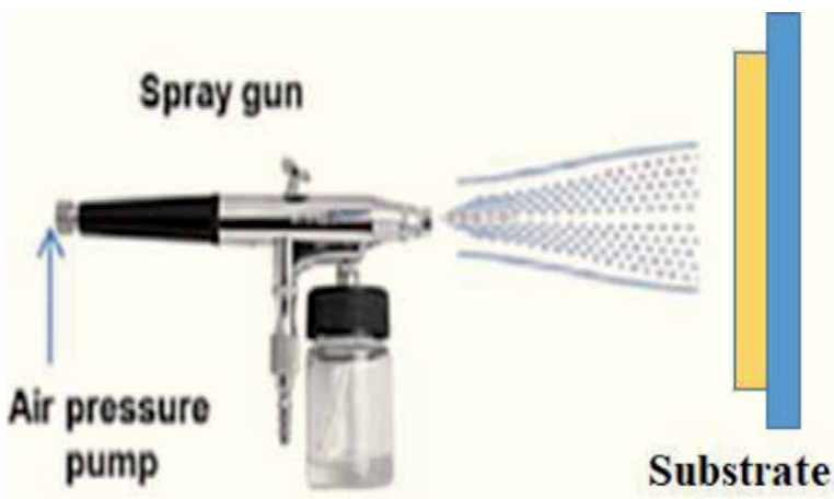
Figure 12. Schematic of the spin-spraying method.
