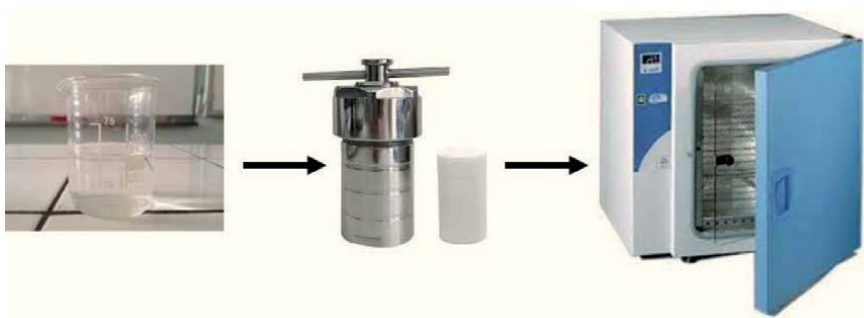
Figure 11. Schematic of the hydrothermal method.
