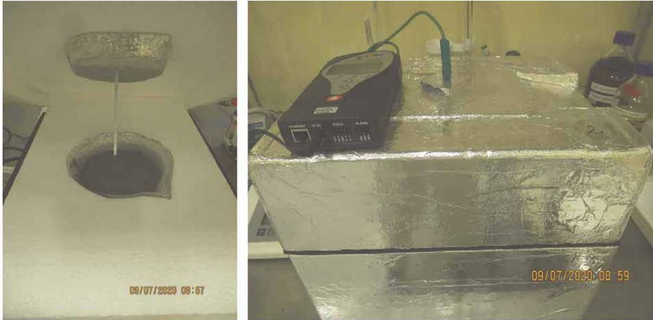
Figure 6. Polystyrene calorimeter with data logger.
