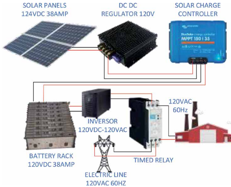
Figure 8. Laboratory power configuration with battery packs.
