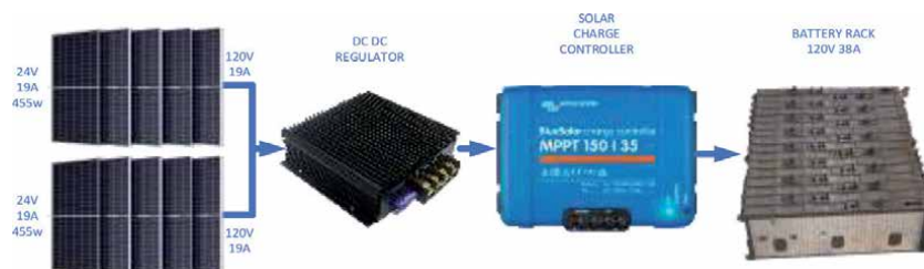
Figure 15. Components of the solar powered charging unit.
