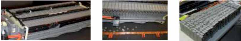
Figure 5. Battery disassembly process.
