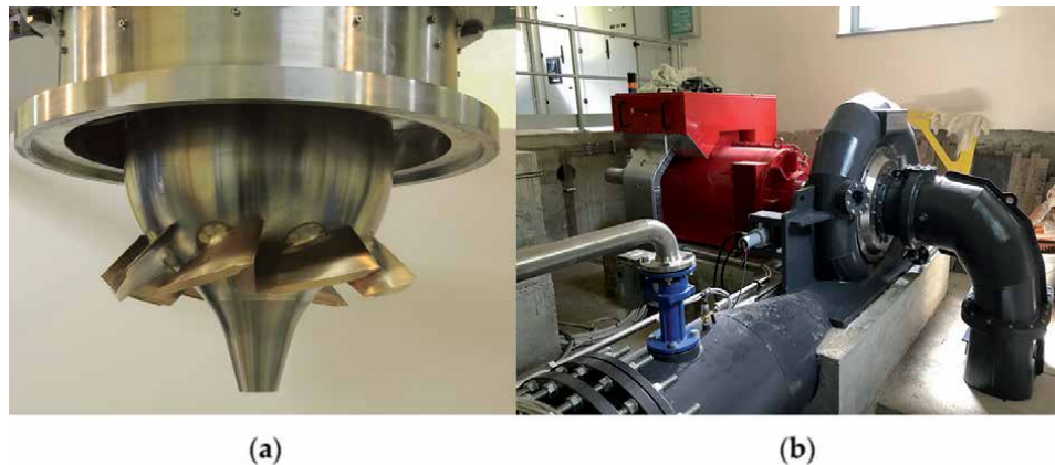
Figure 5. (a) Deriaz turbine (photo courtesy of Mhylab); (b) Deriaz power plant in Italy (photo courtesy of Artingegneria).
