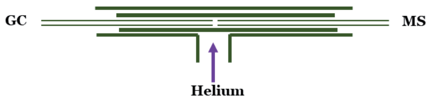
Figure 2. Schematic representation of an open-coupling system.
