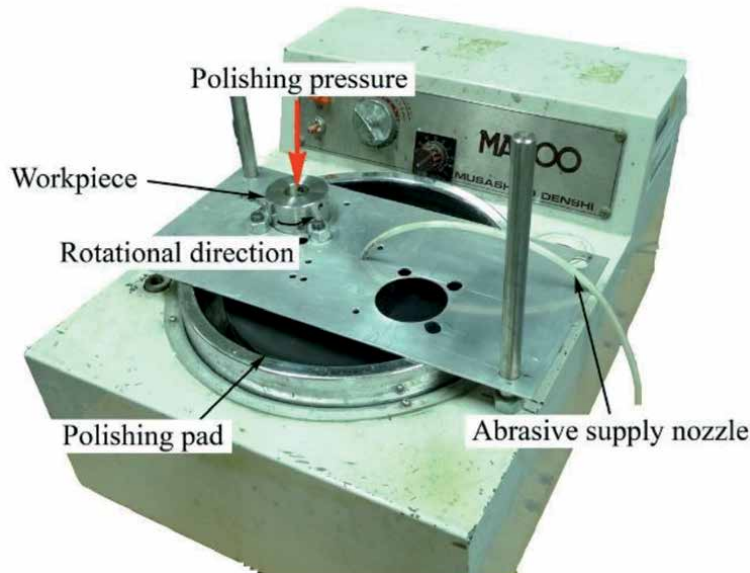
Figure 3. Overview of precision polishing machine and experiment.
