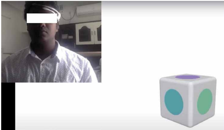
Figure 6. The object movement test of the subject, live mode in BCI App when the person thinks of moving the object left from neutral, the cube has moved left.
