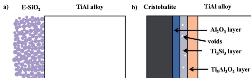
Figure 7. Representation of a \gamma -TiAl alloy coated with E- SiO_2 film (a) and after thermal oxidation test (b) [157].
