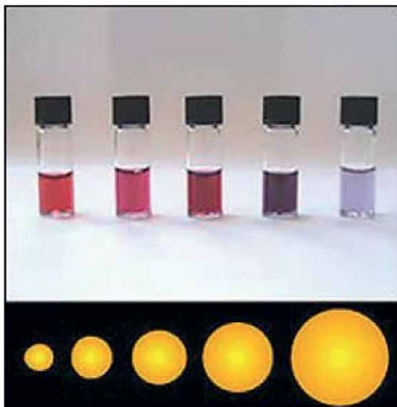
Figure 2. Variations in color of gold nanoparticle suspension as particle size increases. Synthesized gold nanoparticles tend to have wine-red color (average size of 10–15 nm) and turns blue to purple as particles aggregate and get bigger.
