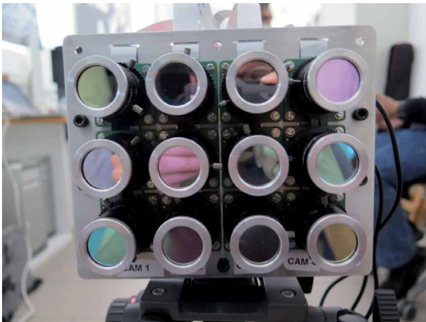
Figure 11. Optical filter detail for hyperspectral camera.
