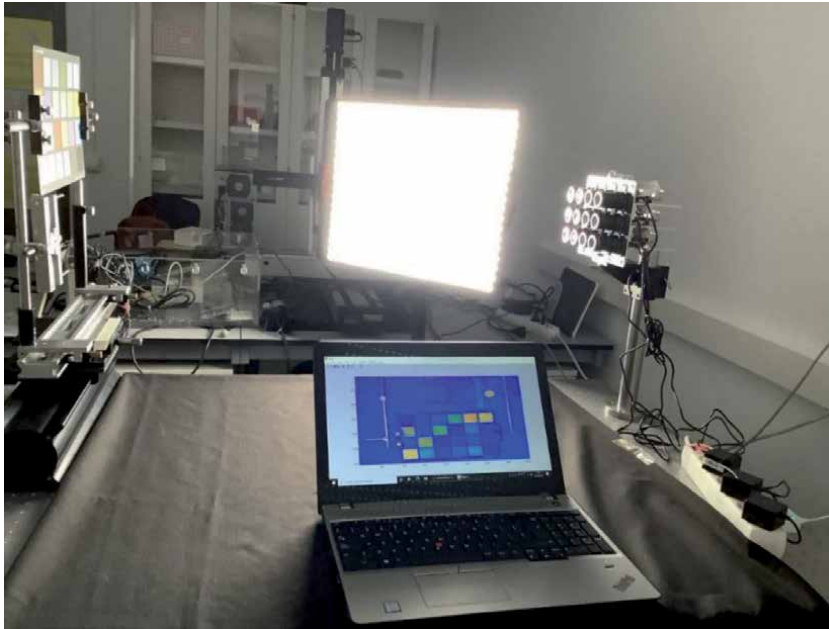
Figure 12. Hyperspectral CCD calibration procedure.
