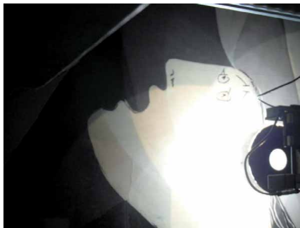
Figure 4. Annular ring source for 35° lighting with a hole in the central area for spectroradiometric measurement.
