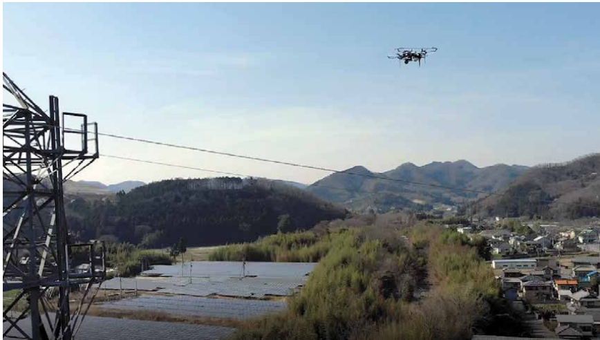
Figure 7. Quadrotor system during power line autonomous inspection.
