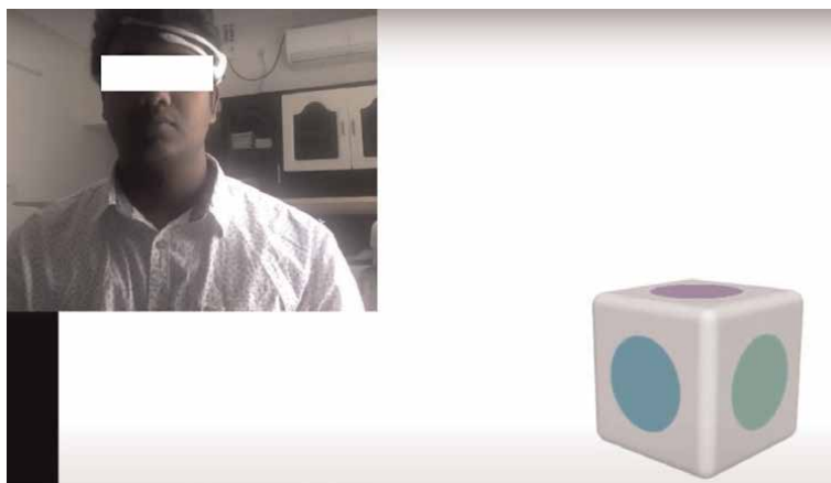
Figure 6. The object movement test of the subject, live mode in BCI App when the person thinks of moving the object left from neutral, the cube has moved left.
