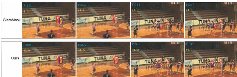
Figure 11. Qualitative comparison between SiamMask and developed data-augmentation technique for incorporating low-resolution datasets during training. Where blue: Ground truth, red: Tracking result.
