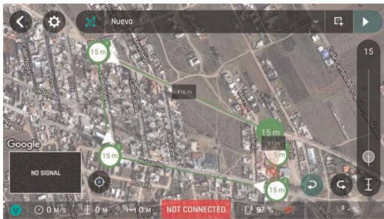
Figure 7. Simulation of a programmed route at 15 m/s.
