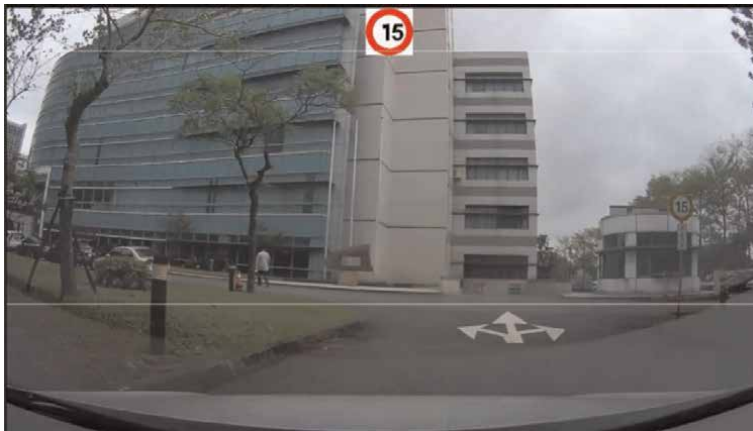
Figure 38. The detection and recognition result of speed limit ending with the digit '5'.
