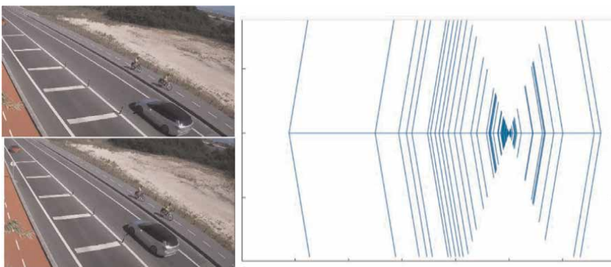
Figure 3. (a) Left side: vehicle shift between moments (t - 1) and t . (b) Right side: representation of the corresponding optical flow.
