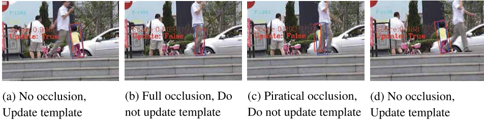
Figure 14. Visual illustration on how the target template update strategy decides whether to update the template or not based on the similarity score under different occlusion scenario during tracking process, VOT2019 girl dataset. Where blue: Ground truth, red: Tracking result.
