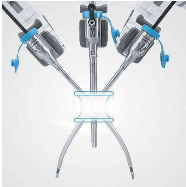
Figure 1. Depiction of robotic arm positioning and orientation with single site surgery.
